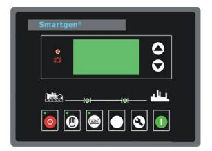
**Standard Control Panel** is the basic configuration for normal operation and usage, adopting deepsea 501K or Automatic Smart-gen 6120 controller (LCD Display). It is of some advantages such as easy to operate, various function and well protection. Operative buttons such as Turn On, Per-heat, Starting, Stop (Emergency Stop) on the panel. While malfunction occurs, control panel will stop the generator and also alarm with light or buzz.
